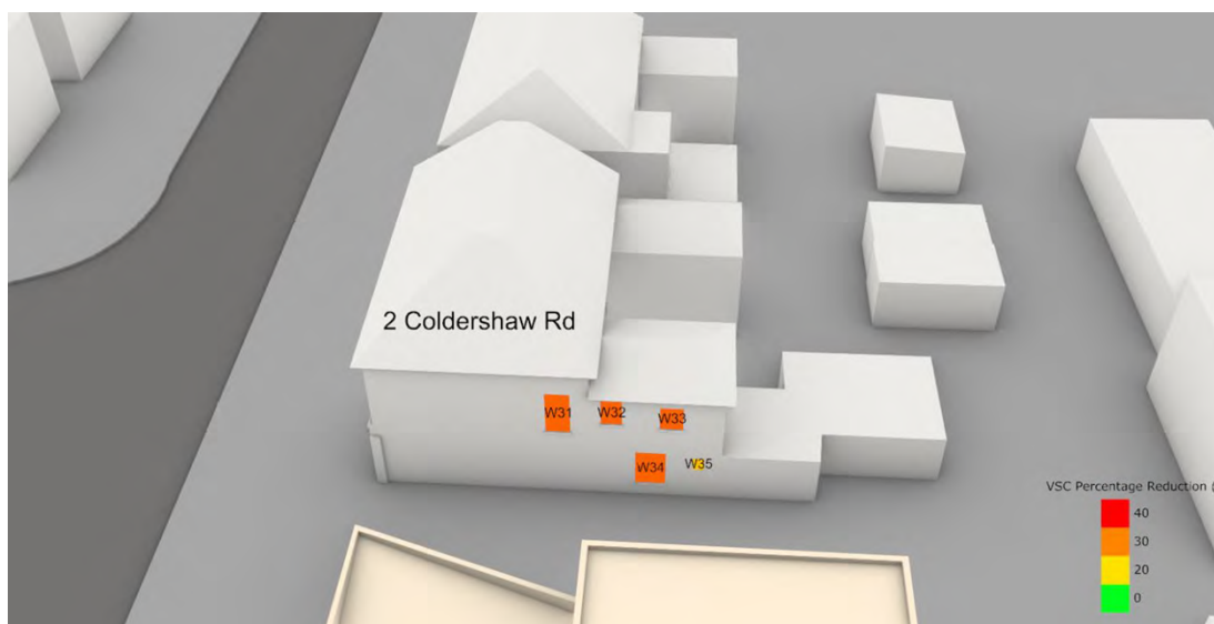
Figure 23 - VSC Magnitude of Impact, window openings at 2 Coldershaw Rd
